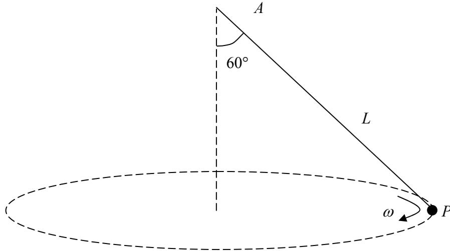
A particle  $P$  of mass  $m$  is attached to one end of a light string. The other end of the string is attached to a fixed point  $A$ . The particle moves in a horizontal circle with constant angular speed  $\omega$  and with the string inclined at an angle of  $60^\circ$  to the vertical, as shown in Fig. 1. The length of the string is  $L$ .
