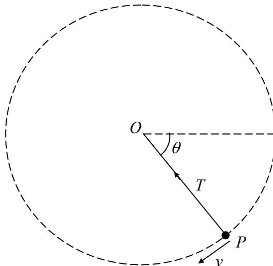
A particle  $P$  of mass  $m$  is attached to one end of a light inextensible string of length  $a$ . The other end of the string is fixed at a point  $O$ . The particle is held with the string taut and  $OP$  horizontal. It is then projected vertically downwards with speed  $u$ , where  $u^2 = \frac{3}{2}ga$ . When  $OP$  has turned through an angle  $\theta$  and the string is still taut, the speed of  $P$  is  $v$  and the tension in the string is  $T$ , as shown in Fig. 3.
