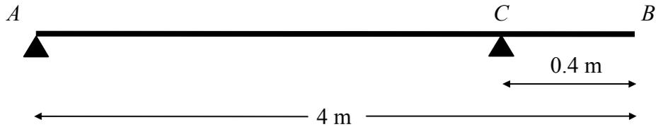
A plank of wood  $AB$  has mass 10 kg and length 4 m. It rests in a horizontal position on two smooth supports. One support is at the end  $A$ . The other is at the point  $C$ , 0.4 m from  $B$ , as shown in Figure 2. A girl of mass 30 kg stands at  $B$  with the plank in equilibrium. By modelling the plank as a uniform rod and the girl as a particle,
