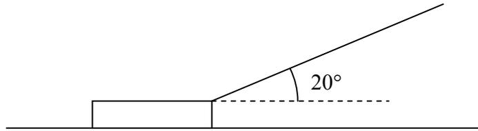
A sledge has mass 30 kg. The sledge is pulled in a straight line along horizontal ground by means of a rope. The rope makes an angle  $20^\circ$  with the horizontal, as shown in Figure 3. The coefficient of friction between the sledge and the ground is 0.2. The sledge is modelled as a particle and the rope as a light inextensible string. The tension in the rope is 150 N. Find, to 3 significant figures,
