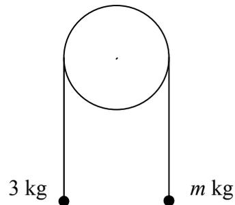
The particles have mass 3 kg and  $m$  kg, where  $m < 3$ . They are attached to the ends of a light inextensible string. The string passes over a smooth fixed pulley. The particles are held in position with the string taut and the hanging parts of the string vertical, as shown in Figure 1. The particles are then released from rest. The initial acceleration of each particle has magnitude  $\frac{3}{7}g$ . Find
