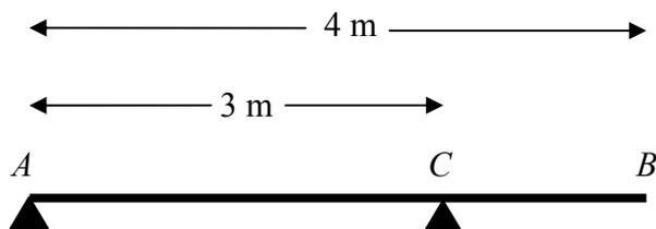
A uniform plank  $AB$  has mass 40 kg and length 4 m. It is supported in a horizontal position by two smooth pivots, one at the end  $A$ , the other at the point  $C$  of the plank where  $AC = 3$  m, as shown in Fig. 1. A man of mass 80 kg stands on the plank which remains in equilibrium. The magnitudes of the reactions at the two pivots are each equal to  $R$  newtons. By modelling the plank as a rod and the man as a particle, find
