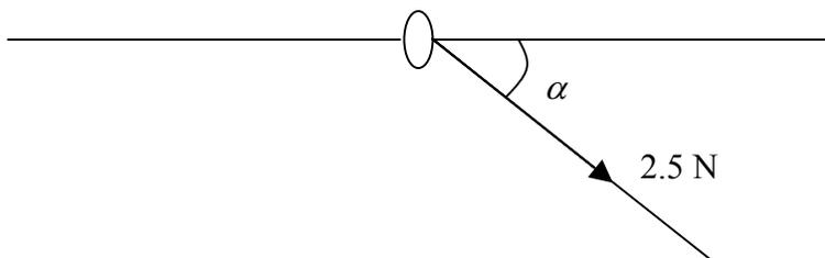
A ring of mass 0.3 kg is threaded on a fixed, rough horizontal curtain pole. A light inextensible string is attached to the ring. The string and the pole lie in the same vertical plane. The ring is pulled downwards by the string which makes an angle  $\alpha$  to the horizontal, where  $\tan \alpha = \frac{3}{4}$  as shown in Fig. 2. The tension in the string is 2.5 N. Given that, in this position, the ring is in limiting equilibrium,
